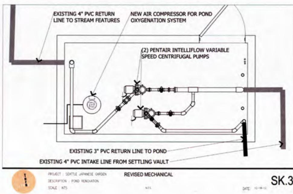
Intelliflo Pump Installation Schematic - 2014
